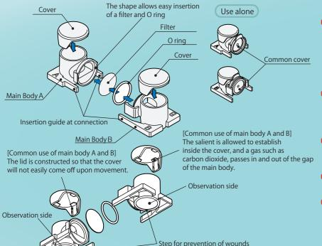
The main body comprises two parts, A and B, and can use the main body cover with the common cover. The common cover prevents the culture medium from spilling on the simple
