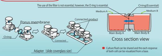
As for the adapter, an existing observation instrument is available for object glass size
