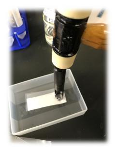
Take care not to scratch the experiment desk even if it punches out too much using the lid of the chip holder etc. Punch out with a hammer. First you need a knack, but it is easy if you get used to it.
