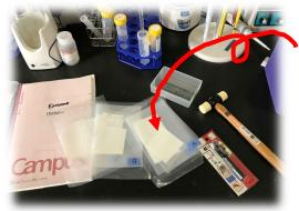
In our co-culture vessel, a circular filter with a diameter of 13 mm is standard, but if you want to use a filter other than 13 mm, adjust the size using a punch. Please purchase a commercially available punch 13 mm diameter. Please use Punch after cleaning and alcohol sterilization.
